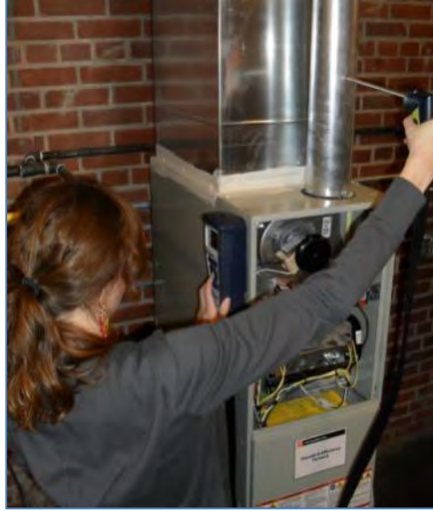
Figure 4. Draft pressure testing using combustion analyzer
