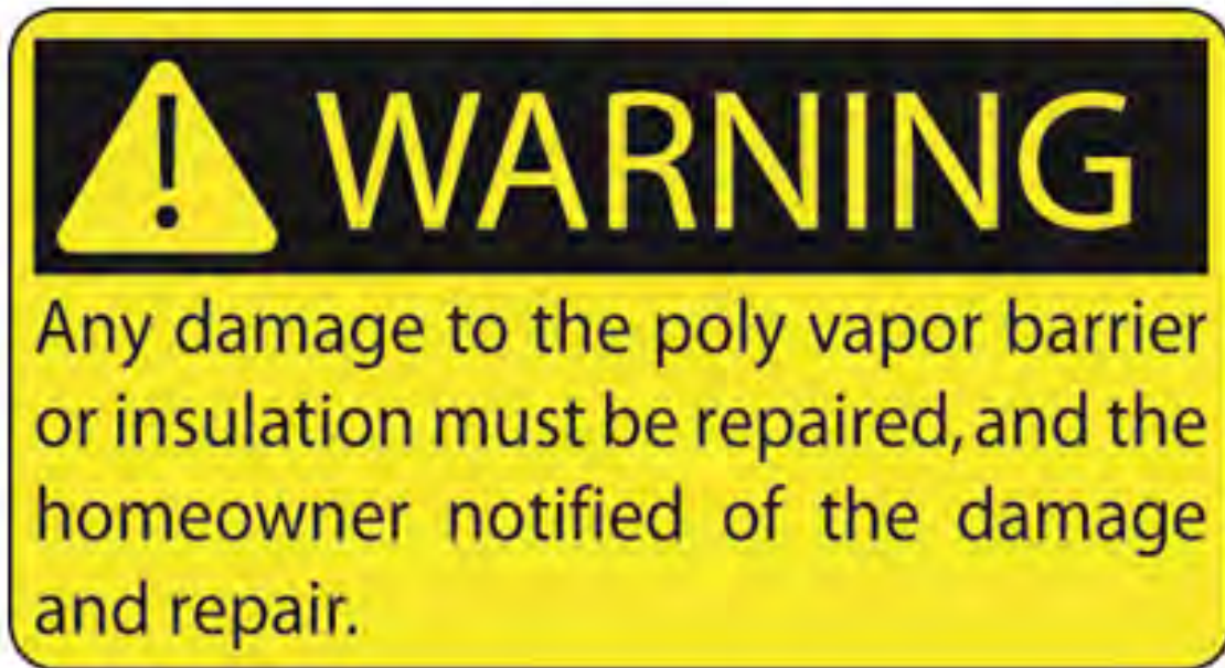
Figure 32. Example of a warning sign posted at an access entryway
