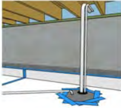
Figure 25. Crock pit lid sealing
