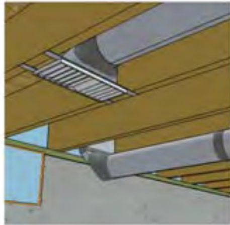
Figure 13. Supply air diffuser
