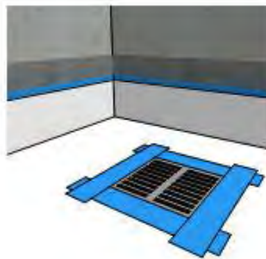
Figure 26. Low-point floor drain sealing
